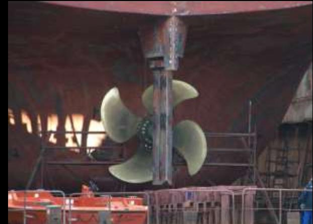
Due to the position of the ship's propeller above the hull bottom of the ship, a sound shadow is created on the bow side
